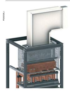
Switchboards can be equipped with connections for Canalis KT. Jointing with the switchboard is via a standard run component (straight length, elbow, etc.) and a jointing unit (identical to those used between line components). The trunking enters the switchboard via the top (roof).
