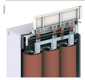
Canalis KT can be connected to cast resin transformers using a universal feed. The connection is made using a flexible busbar (connection plates or braids) to avoid transmitting vibrations and expansions. The connection plates are made up of either insulated or non-insulated flexible copper bars, drilled at one or both ends. A nut and bolt kit allows connection to the feed.
