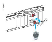
The junction between sections is made using a joint block.
